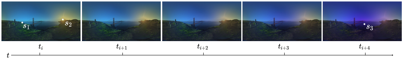
Figure 4. Visualization of parameter interpolation. Spatial keyframes s_1 (cyan) and s_2 (yellow) at time t_i and s_3 (purple) at time t_{i+4} , interpolate both spatially and temporally using radial basis functions. Note this does not represent the in-headset viewing experience because any single pixel will have different parameters applied to it depending on the users’ view.
