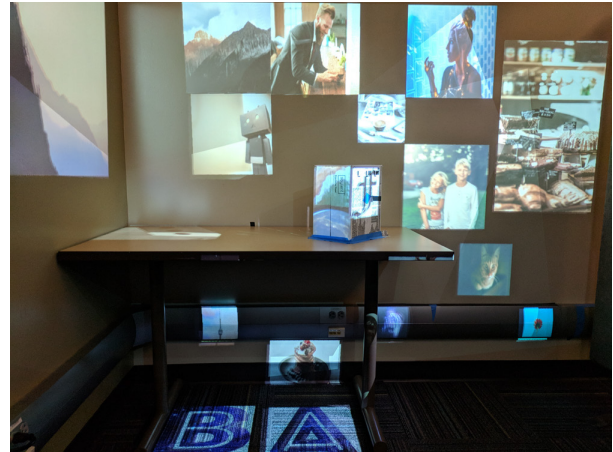
Figure 4: An example of spatial content viewed in the SAR setup. Note how content can be displayed on any surface including walls, floor, furniture, and objects.
