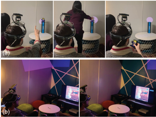
Figure 6. Ambient display examples: (a) spotlight as a contextual environment display; (b) mood-lights as ambient environment lighting
