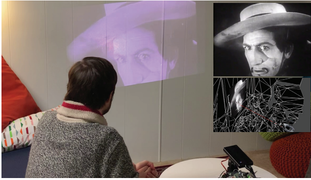
Figure 2. AR persistence example application. The projector acts as an ad hoc display when the user takes off the HMD, enabling them to continue watching a video started in AR.
